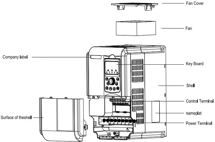
Figure 1.3 Components of Plastic Case Model
