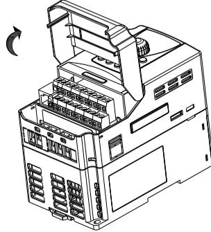
Figure 2.2 Remove the Cover Plate (Plastic Case)
