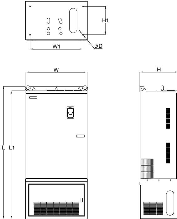
Figure 1.8 Cabinet Installation Dimensions
