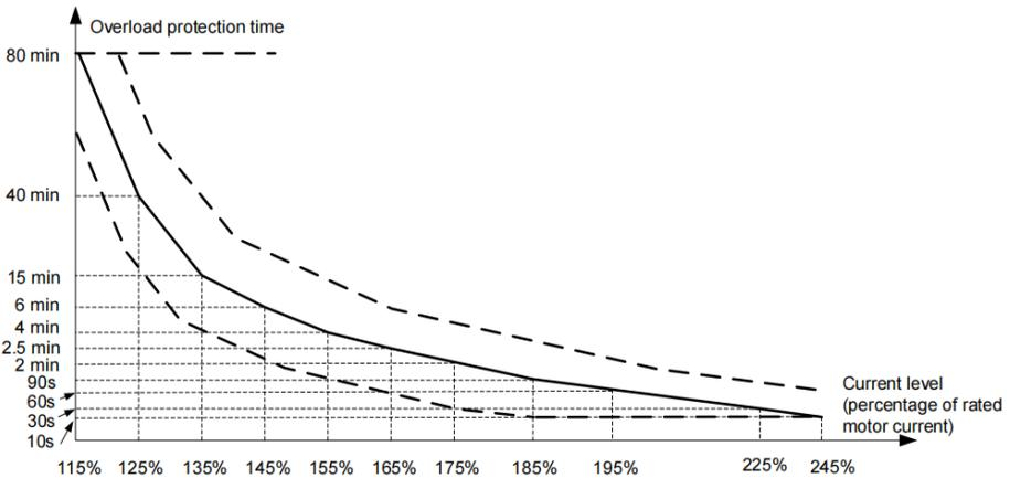
When motor running current reaches 175% of rated motor current and motor runs at this level for 2 minutes, Err11 (motor overload) is detected. When motor running current reaches 115% of rated motor current and motor runs at this level for 80 minutes, Err11 is detected.
