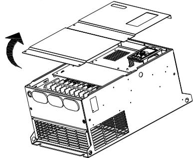
Figure 2.3 Remove the Cover Plate (Metallic Case)
