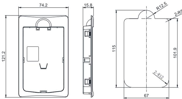
Figure 1.10 Keyboard Tray Appearance and Hole Size (mm)
