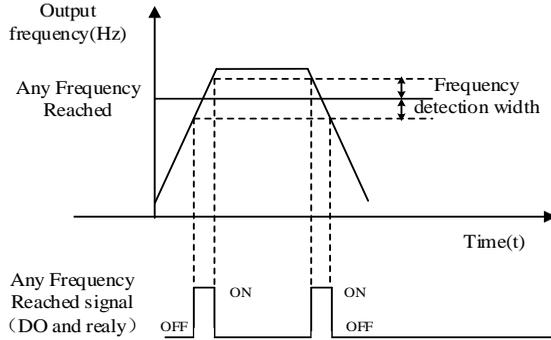
If the output frequency of the inverter is within the positive and negative amplitudes of the any frequency reaching detection value, the corresponding digital output becomes ON.
