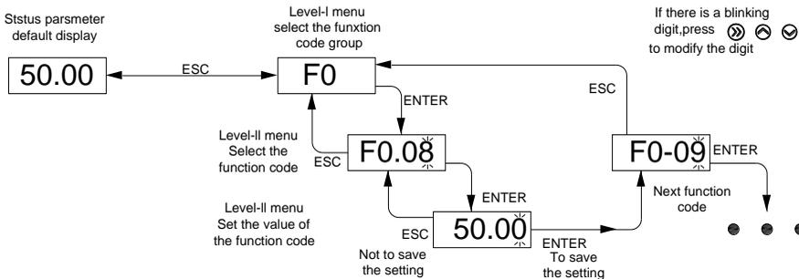
Figure 4.3 Three-Level Menu Float Chart of Operation Procedure
