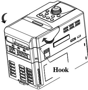
2. Lift the cover to open the inverter.
