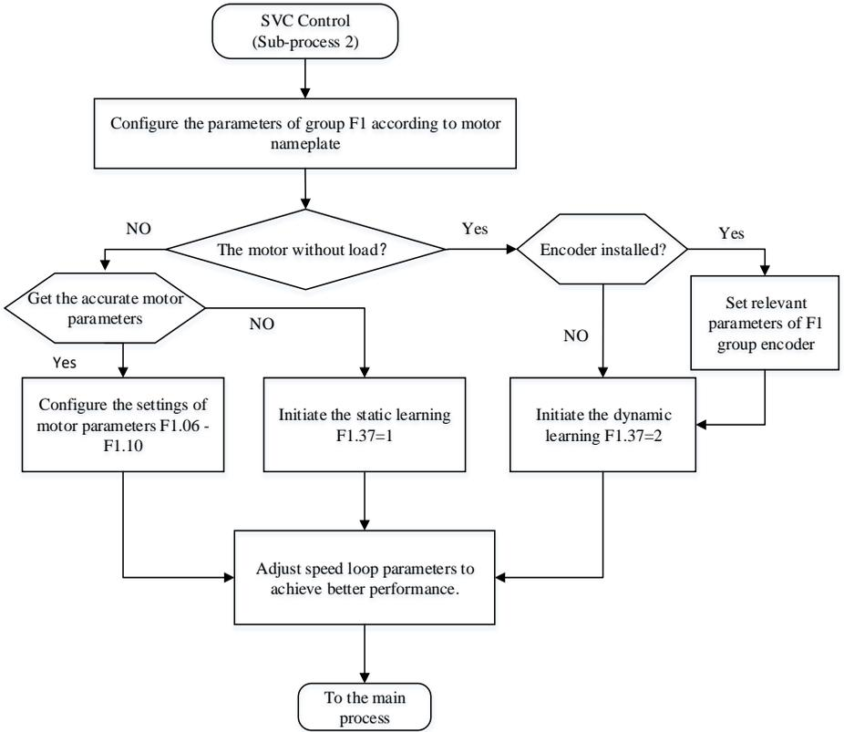
Figure 5.3 Inverter's Adjustment Sub-Process Flow (Vector Control)
