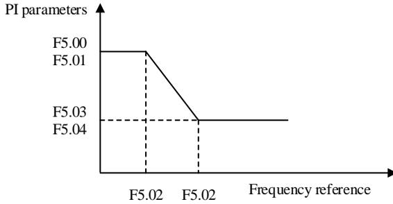
To improve the system response, increase the proportional gain or reduce the integral time. Remember to increase proportional gain first to ensure that the system does not oscillate, and then reduce integral time to ensure that the system has quick response and small overshoot.
