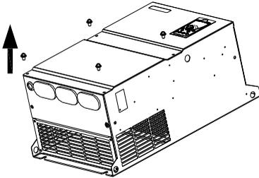
2. Lift the cover to open the inverter.
