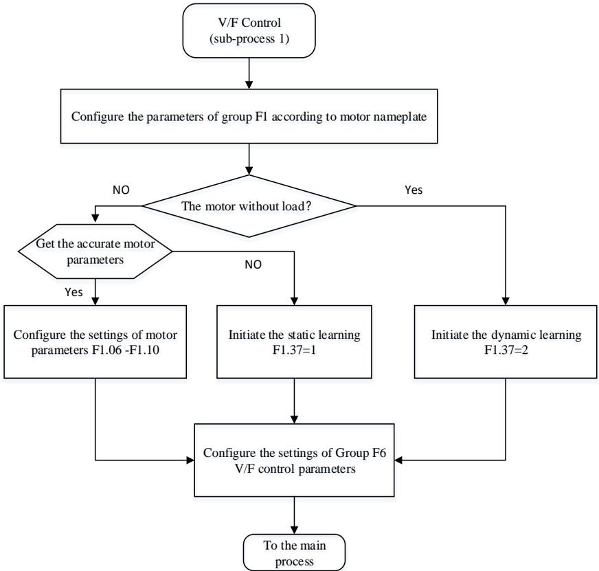
Figure 5.2 Inverter's Adjustment Sub-Process Flow (V/f Control)
