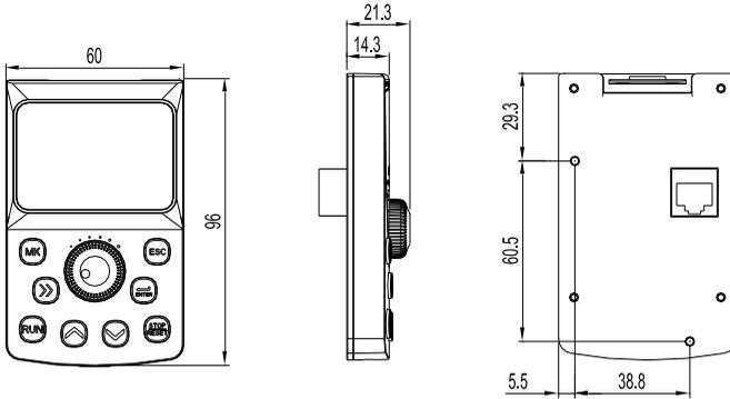
Figure 1.9 Appearance and Dimensions of the Keyboard (mm)
