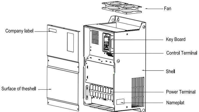
Figure 1.4 Components of the Metallic Case Model
